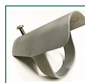
5° Tilt Adjustment Adapter for Spigots. Ensures that correct tilt can be achieved if the original pole outreach angle is incorrect. Factory fitted. Can in some instances be site fitted. See your Roadway & Infrastructure Sales Representative for advice.
