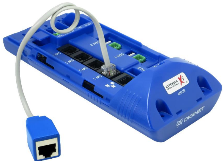
Connection between the eHub and RJ-45 patch lead
